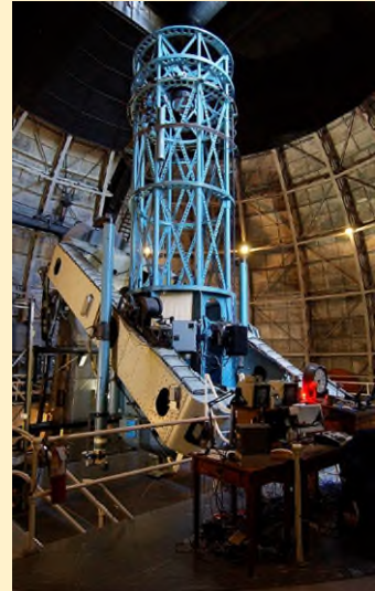
Hooke 100" telescope at Mount Wilson, used by Edwin Hubble, Wikipedia CC by 3.0
